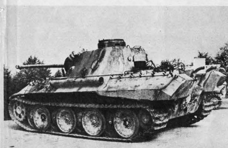
Germany's continued interest in the overlapping-wheel design for track support is evident in her newest tanks, PzKw V Panther (above) and the PzKw VI Tiger at right. Both tanks have eight bogie wheels.
